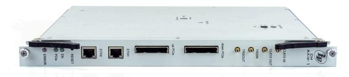
The module is designed to operate as part of measuring systems created on the basis of the AXIe-1 trunk. The module acts as a system module of the AXIe-1 standard chassis.
